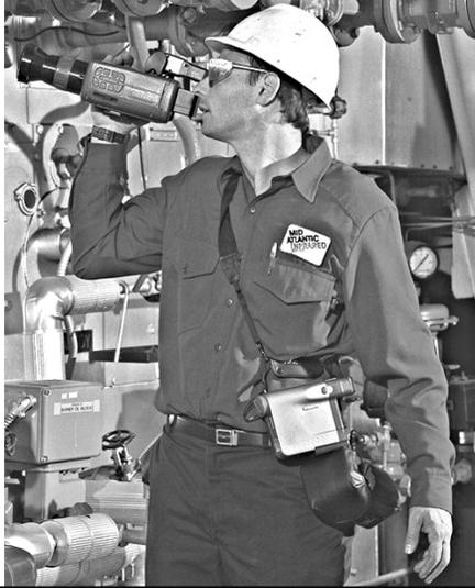
**Figure 1: Inframetrics Thermo-cam, digital camera and lenses**
