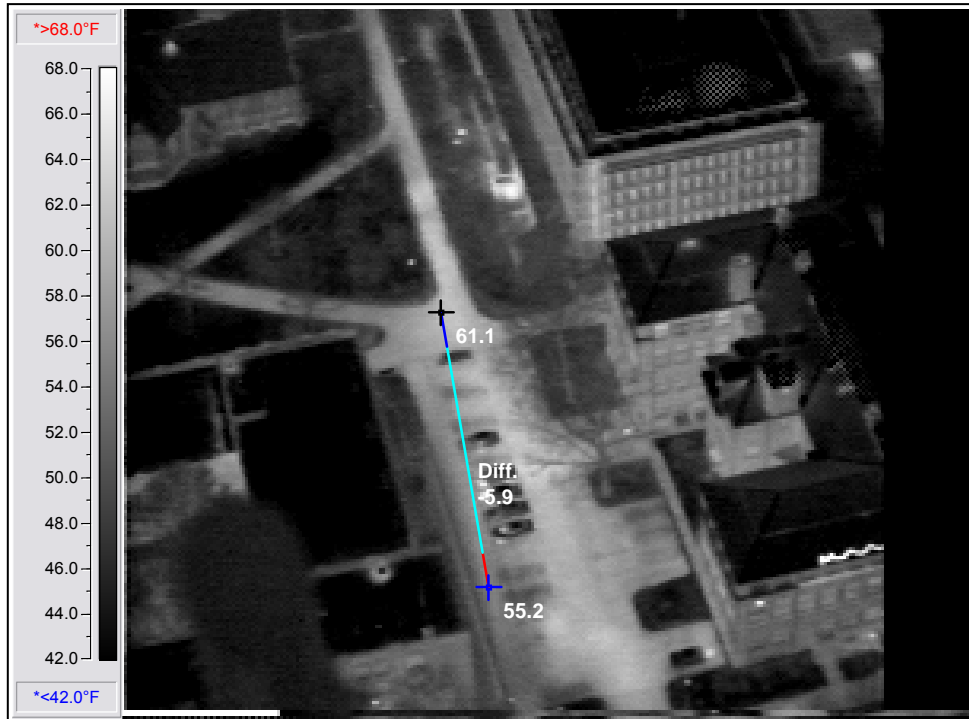
Comparative 2005 image. No heating is seen at the location of the current suspected leak. Note: Image angle is reversed 180° from present image.
