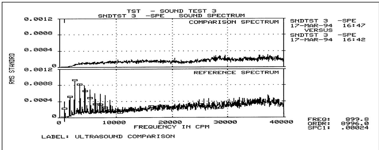
The next case was produced from a screw conveyor. The rotational speed of the conveyor was 66 CPM. The conveyor produced an audible grind. The demodulated ultrasound spectrum shows an impact occurring once per revolution. The worn drive sheave on the conveyor was replaced, thereby correcting the problem.
