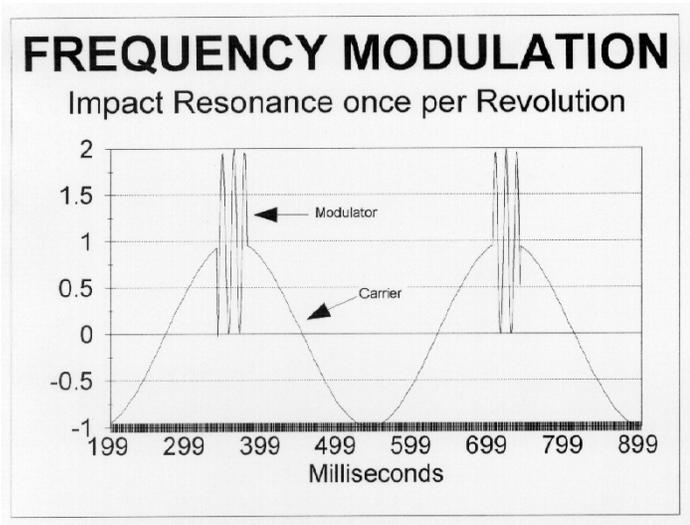
occurs during a "bump test" to determine a resonance. Excited high frequency vibration is represented in the example drawing by the waveform marked "Modulator". Thus, the resonant vibration resulting from the once per revolution impact is modulating the once per revolution signal. The demodulated signal in this case will return just the carrier. It will indicate the frequency at which the modulating is occurring. That is, it will indicate the frequency at which the impact is occurring.
