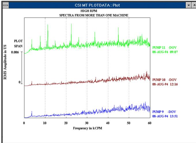
These spectra show that no bearing fault frequencies are visible in the adjacent pumps. Once the pump bearing was changed, the audible buzz disappeared.
